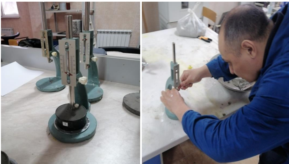
Figure 1 – Determination of the setting time of the dough of standard consistency (beginning and end of setting)
