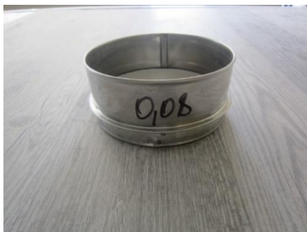
Figure 1 – 0.08 mm sieve for determining cement fineness
