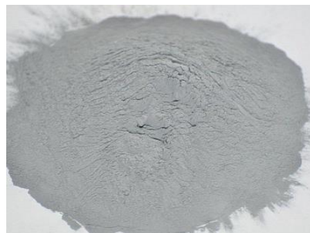
Figure 2 – Portland cement weighing, passed through 0.08 mm sieve
