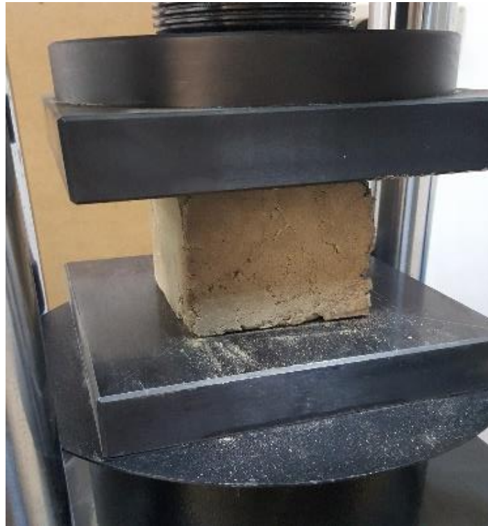
Figure 5 – Hydraulic press testing process
