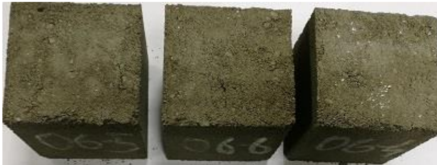
Figure 3 – Samples of cubes after the vibrating table
