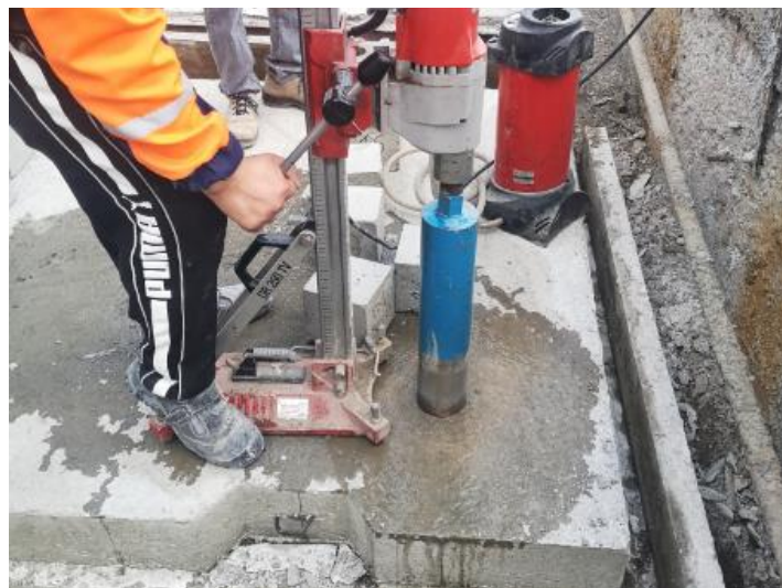
Figure 5 – Process of drilling core samples
