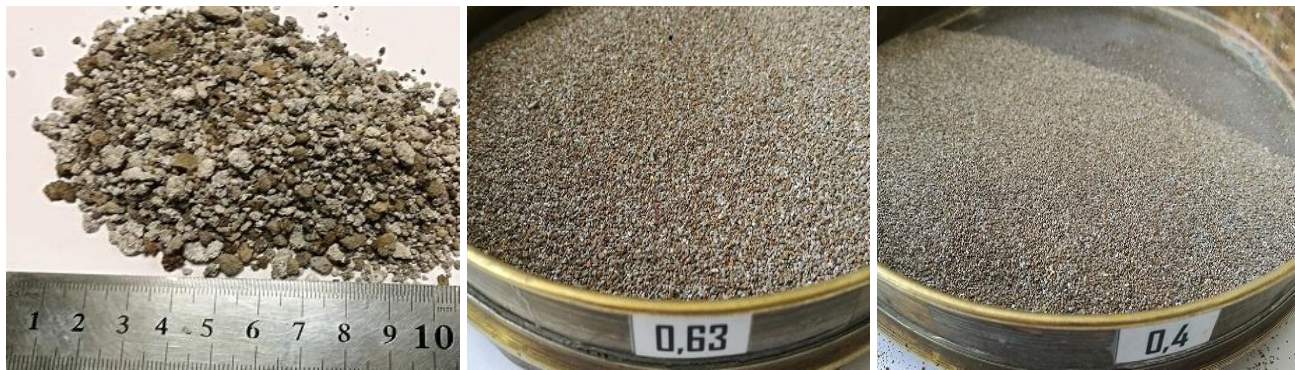
Figure 2 – Bauxite sludge: a) from the Pavlodar Aluminum Plant; b) fraction 0.63; c) fraction 0.4
