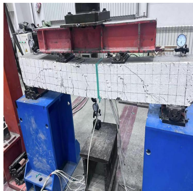
b) Shear failure
