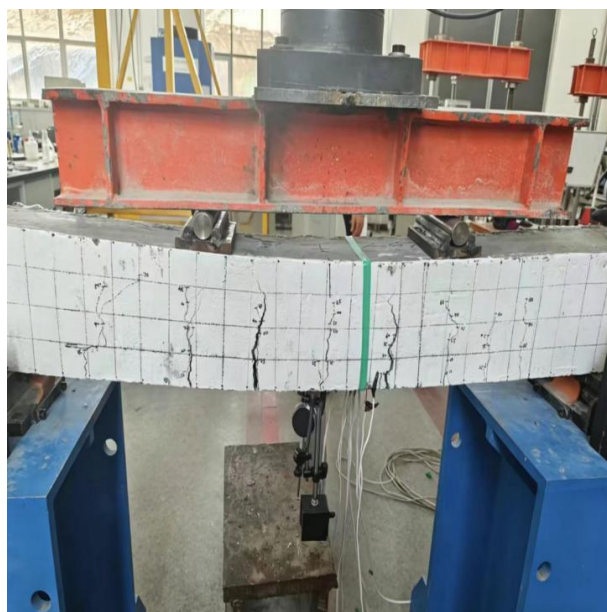
a) Flexural failure
