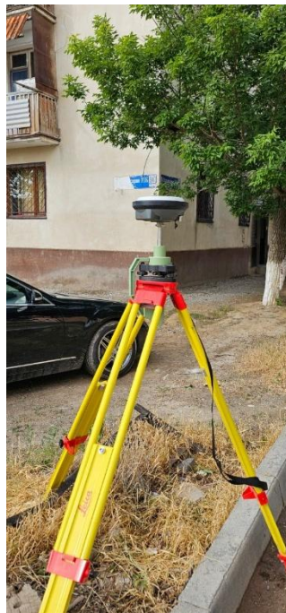
Figure 3 – Temporary GNSS benchmark
