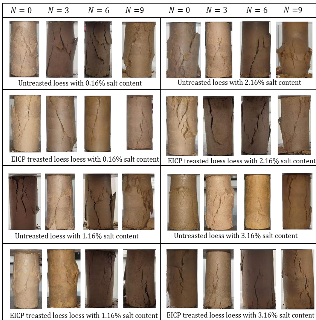
Figure 8 – Failure modes of molded loess specimens after freeze-thaw cycling under UCS testing
