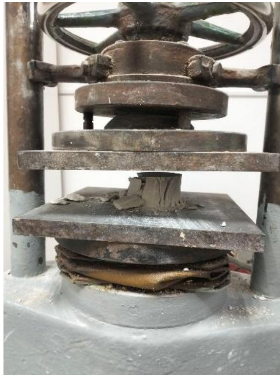
Figure 3 – Compression test of specimens
