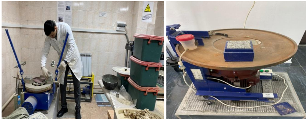
Figure 2 – Testing aerated concrete samples for abrasion resistance
