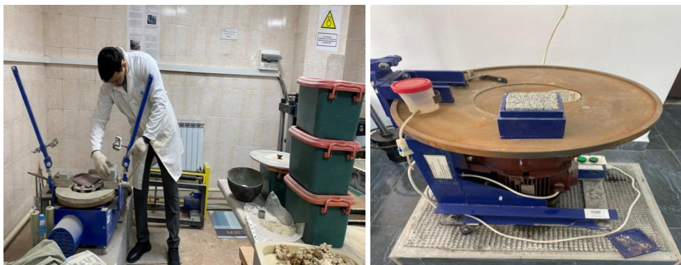
Figure 2 – Testing aerated concrete samples for abrasion resistance
