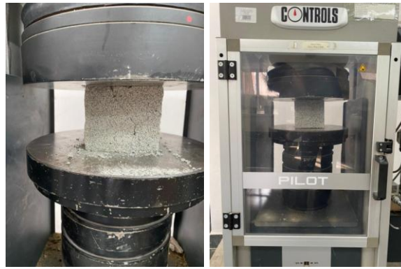
Figure 1 – Testing aerated concrete samples for compressive strength
