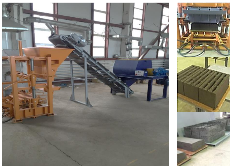
Figure 1 – LWAC blocks manufacture using the “Mastek-Meteor” molding/vibro-pressing complex
