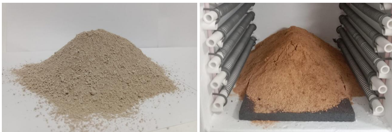
Figure 1 – Finely ground (left) and fired (right) diatomite
