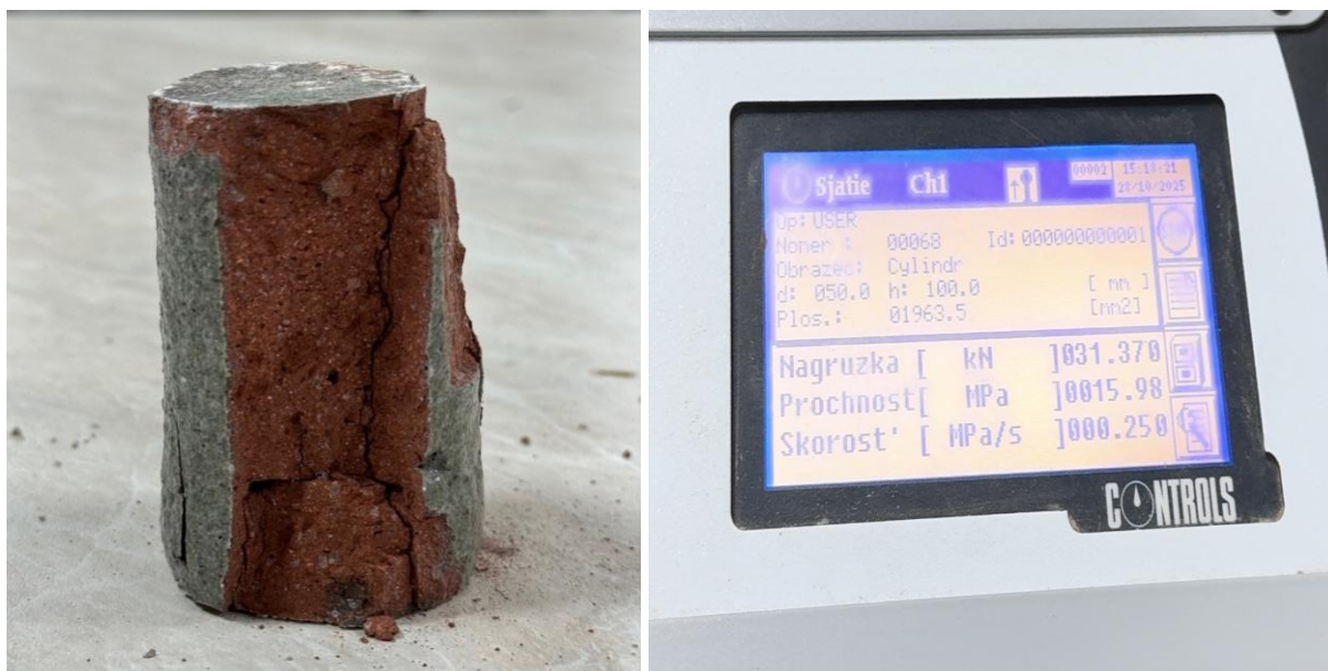
Figure 3 – Ceramic material tested for compressive strength
