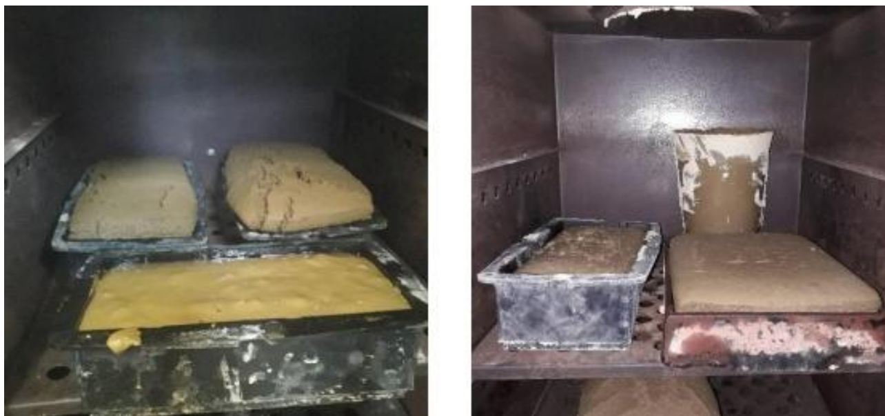
Figure 4 – Slip for gas-ceramic production poured into molds
