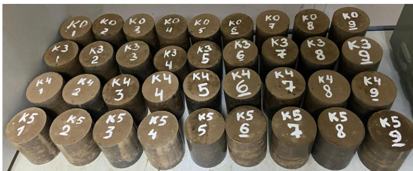
Figure 2 – Cylindrical samples from soil-cement mixes
