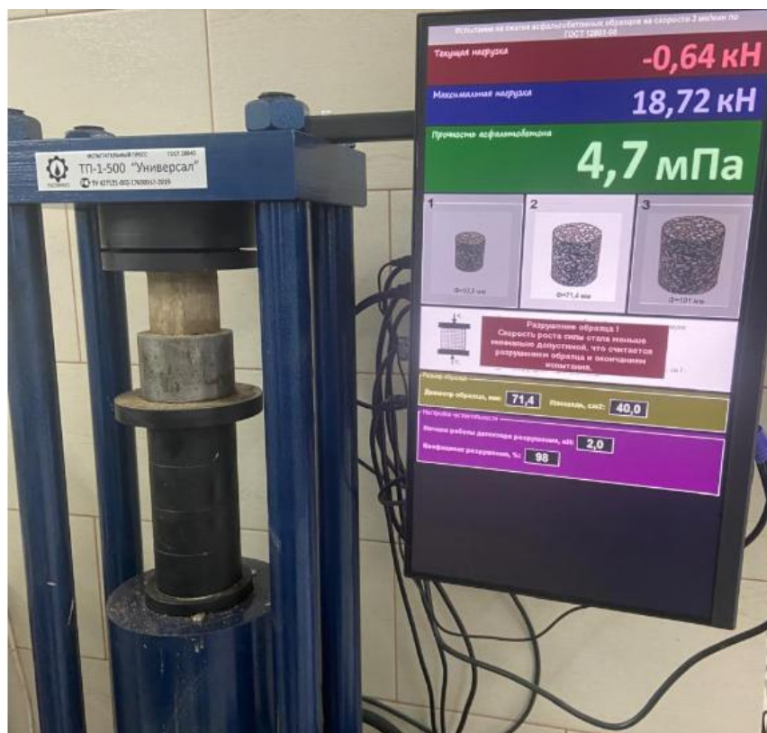
Figure 3 – Determination of the compressive strength of samples
