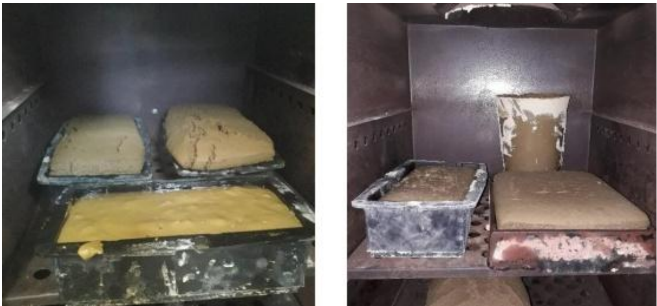
Figure 4 – Slip for gas-ceramic production poured into molds
