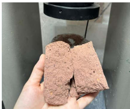
Figure 2 – Ceramic sample tested for compressive strength
