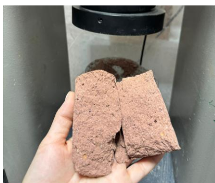
Figure 2 – Ceramic sample tested for compressive strength
