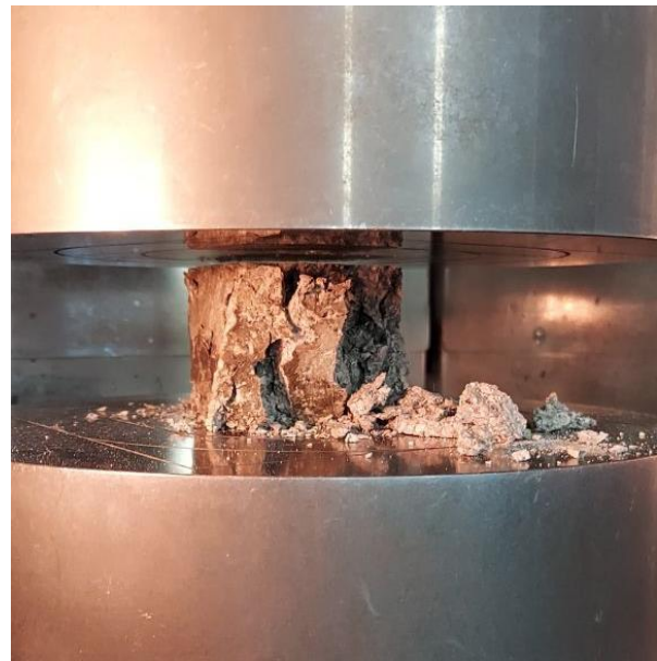
b) Strength test of the specimen with dimensions 50×50×50 mm
