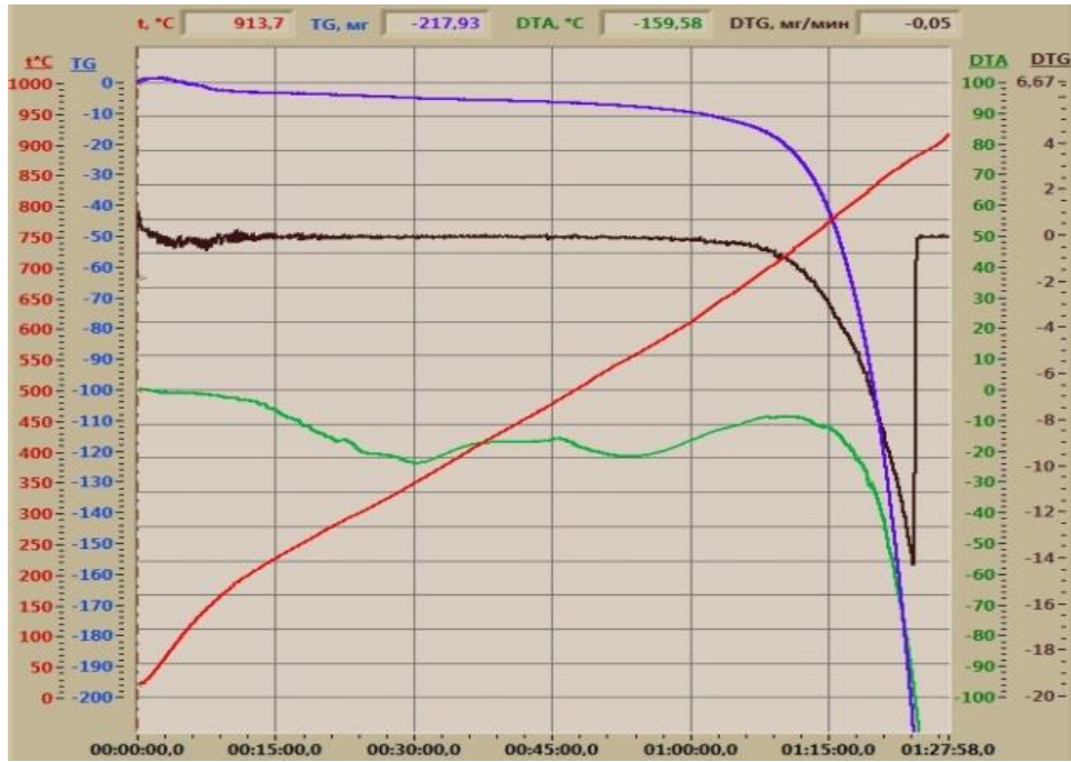
Figure 2 – Results of raster differential thermal analysis of technogenic residues formed during grinding of Sastobe carbonate rocks
