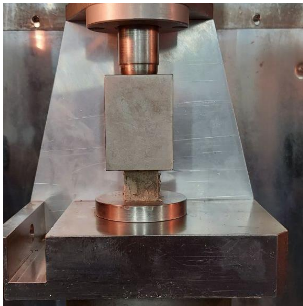
a) Strength test of the specimen with dimensions 20×20×20 mm
