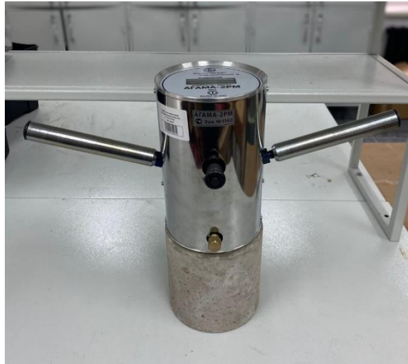
Figure 2 – Determination of water absorption on the AGAMA-2RM device
