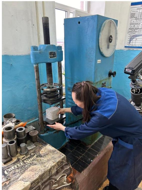
Figure 5 – Mechanical compressive strength test
