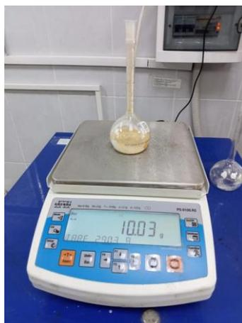
Figure 3 – Determination of sample weight after drying
