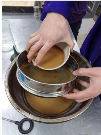
Figure 2 – Washing mineral powder through a 0.063 mm sieve
