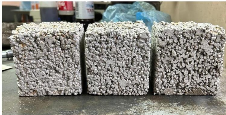
Figure 2 – Polystyrene concrete samples for research
