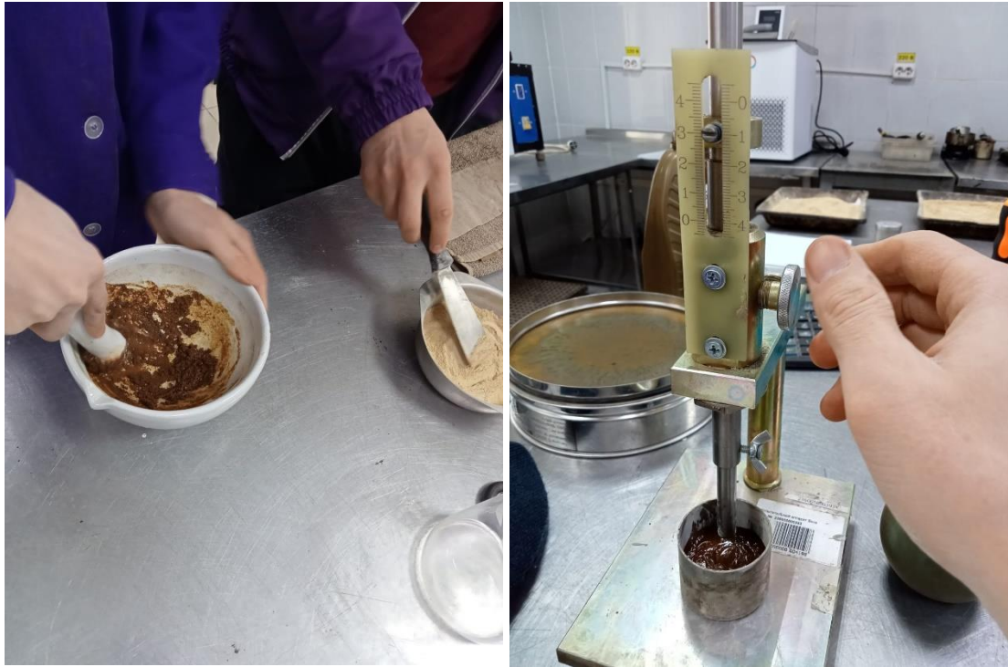
Figure 5 – Determination of bitumen capacity
