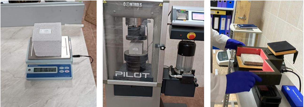
Figure 1 – Laboratory testing of foam concrete
