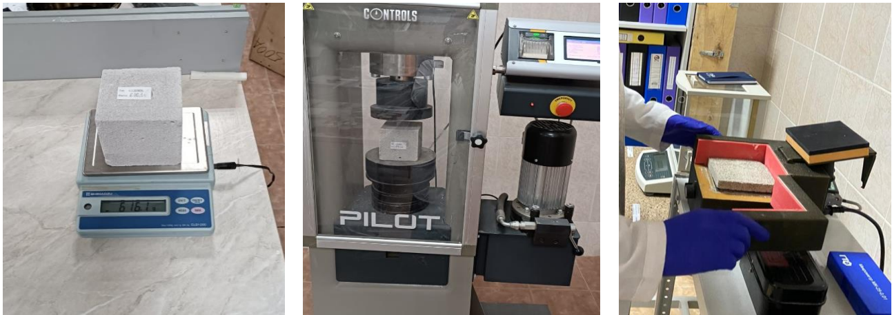
Figure 1 – Laboratory testing of foam concrete
