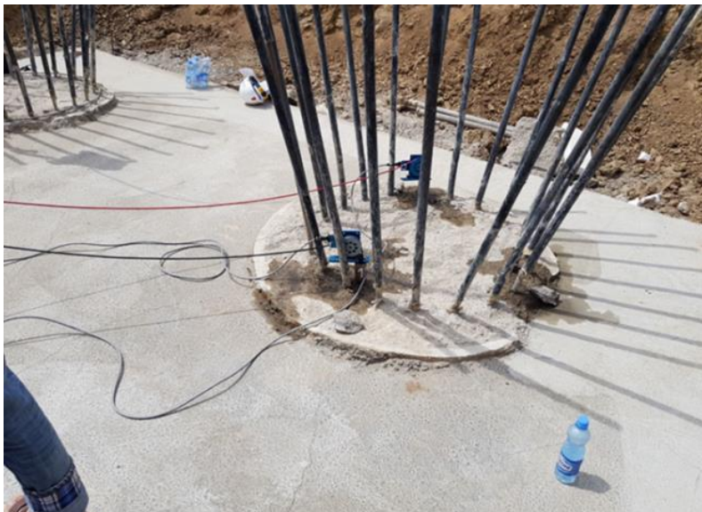
Figure 5 – CSL pile testing with two probes
