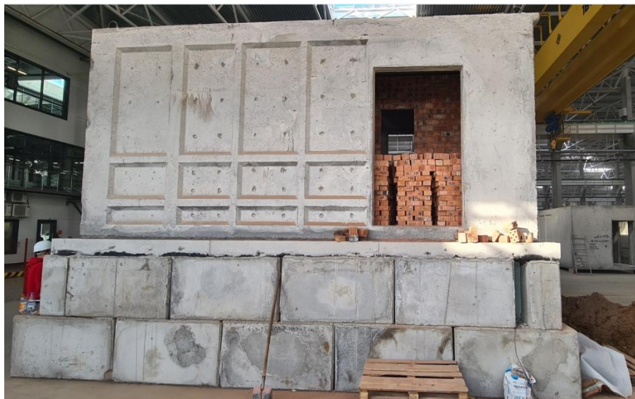
Figure 2 – Loading the ceiling slab with brick columns
