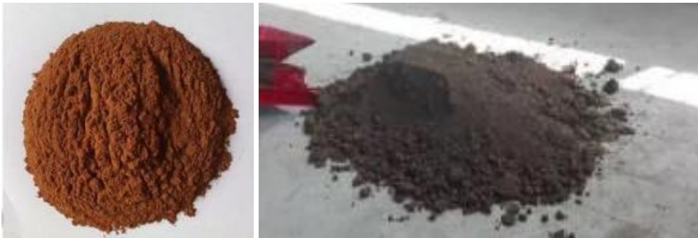
Figure 6 – Clay of Temirtau deposit and mineral wool waste Korolek for preparation of prototypes
