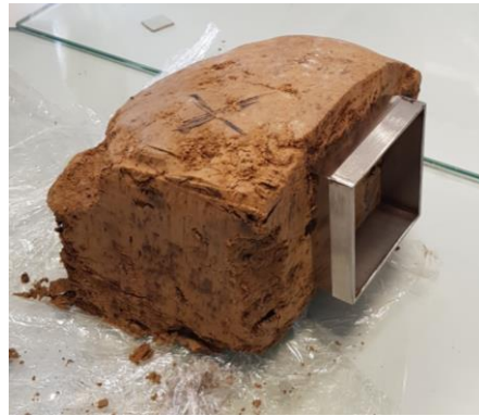
b) Shear direction 90°
