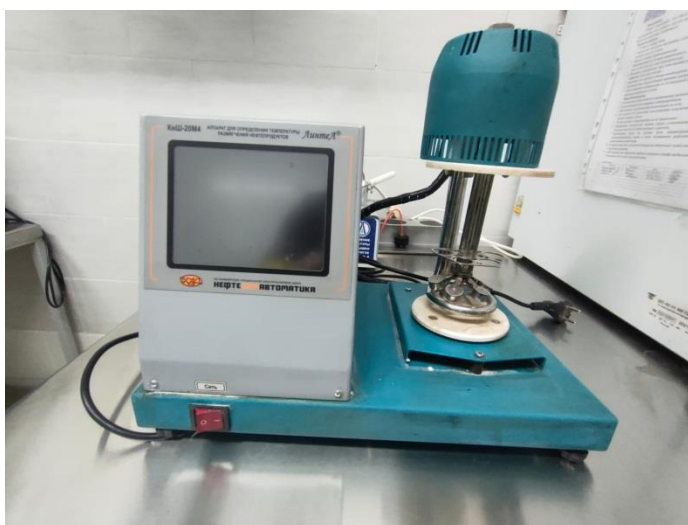
Figure 3 – Determination of bitumen softening temperature on the "ring and ball" device
