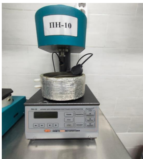
Figure 2 – Determination of bitumen viscosity on penetrometer
