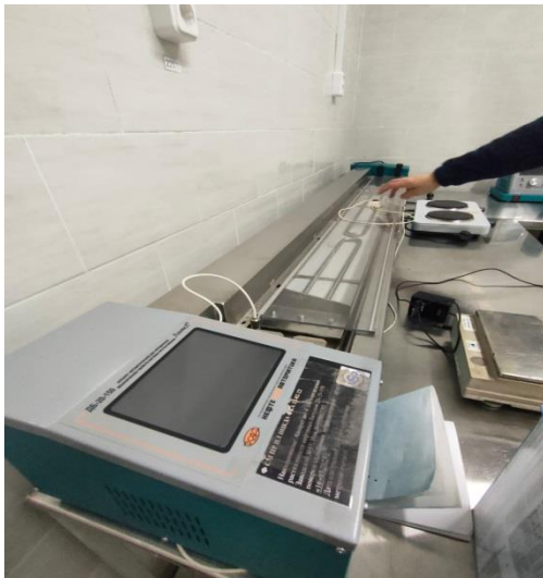
Figure 4 – Determination of bitumen extensibility on a ductilometer
