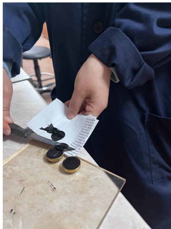
Figure 5 – Cutting of excess bitumen
