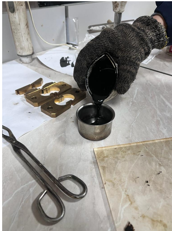
Figure 2 – Pouring bitumen samples into penetration cups
