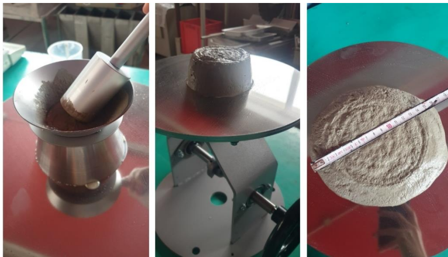
Figure 1 – Testing the freshly prepared mixture to evaluate the needed consistency
