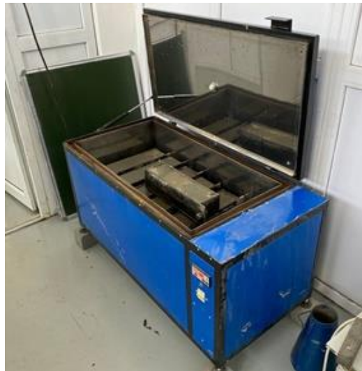
Figure 1 – Universal steaming chamber KUP-1
