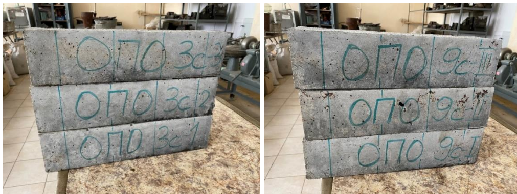
Figure 2 – SFRC samples with vibration times of 3 (left) and 9 (right) seconds
