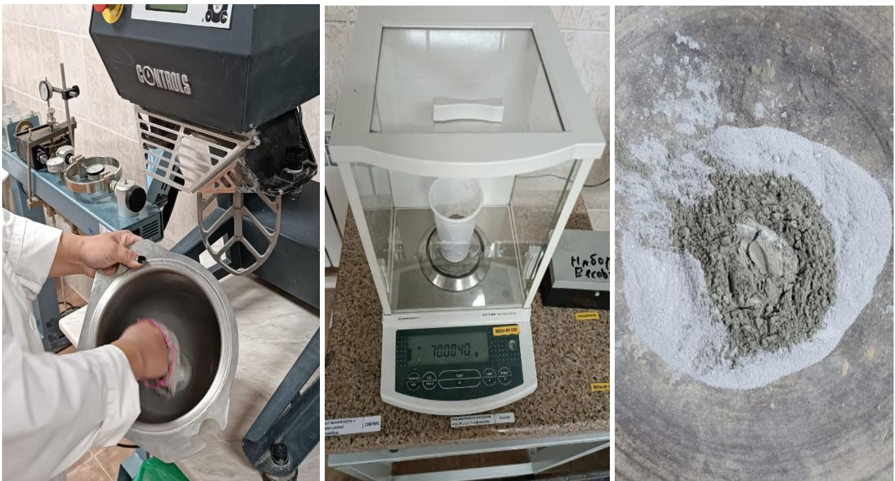
Figure 1 – Sample preparation for XRF and XRF analysis
