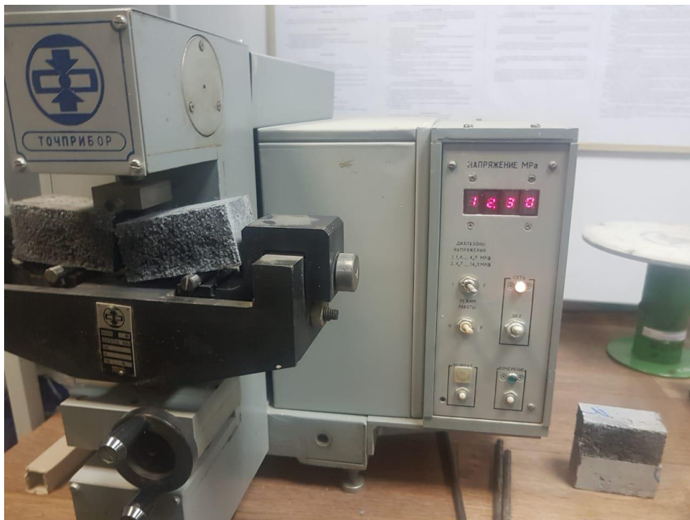
Figure 2 – Bend strength test of the specimen
