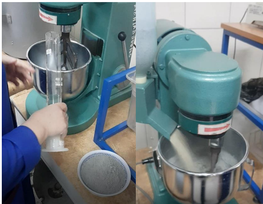
Figure 1 – The steps of preparing the cement dough
