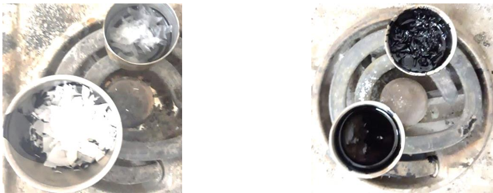
Figure 2 – Mixing bitumen with plastic and polyethylene samples
