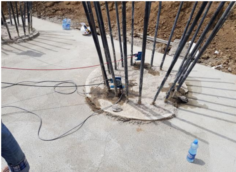
Figure 5 – CSL pile testing with two probes
