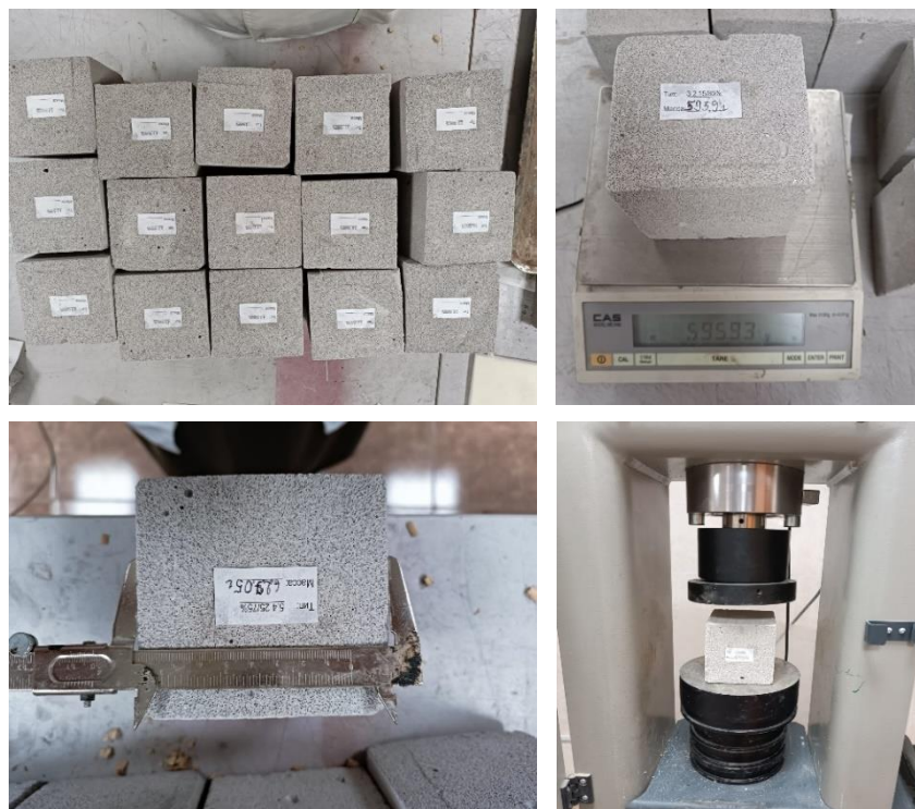
Figure 2 – Laboratory testing of foam concrete samples
