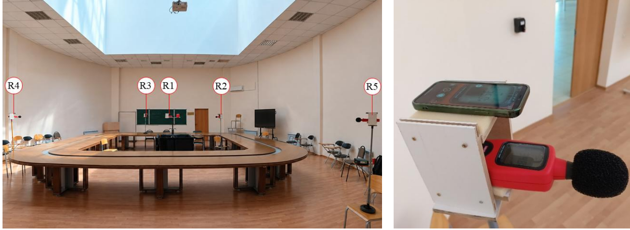
Figure 2 – Measurement setup: R1-R5 – receivers
