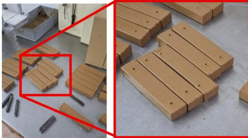
Figure 2 – Prepared samples of building ceramics before drying and firing
