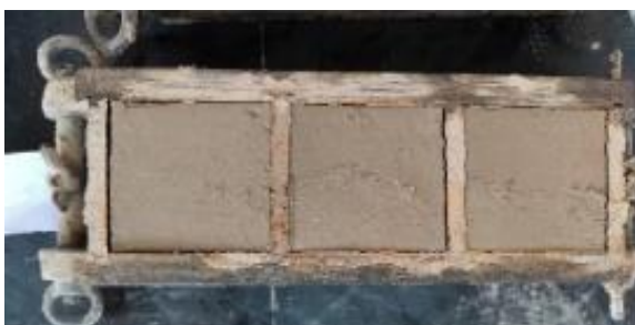
a) Gap appearing between the specimen and the mold
