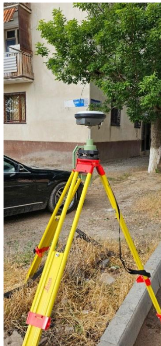
Figure 3 – Temporary GNSS benchmark
