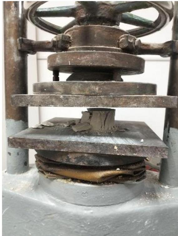
Figure 3 – Compression test of specimens
