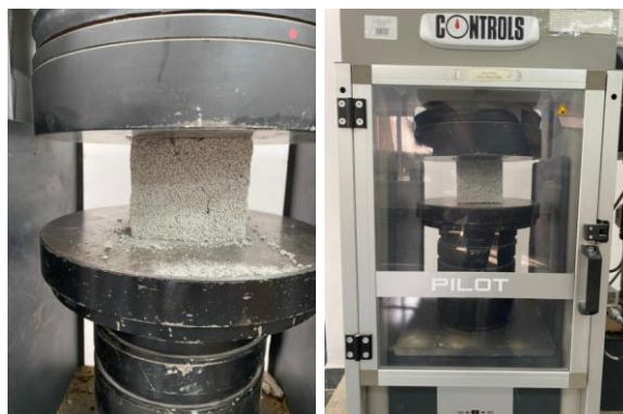
Figure 1 – Testing aerated concrete samples for compressive strength
