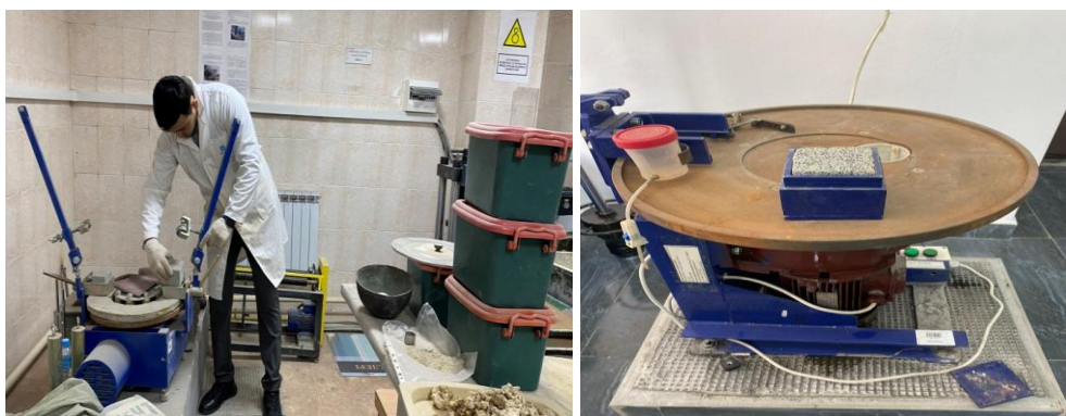
Figure 2 – Testing aerated concrete samples for abrasion resistance
