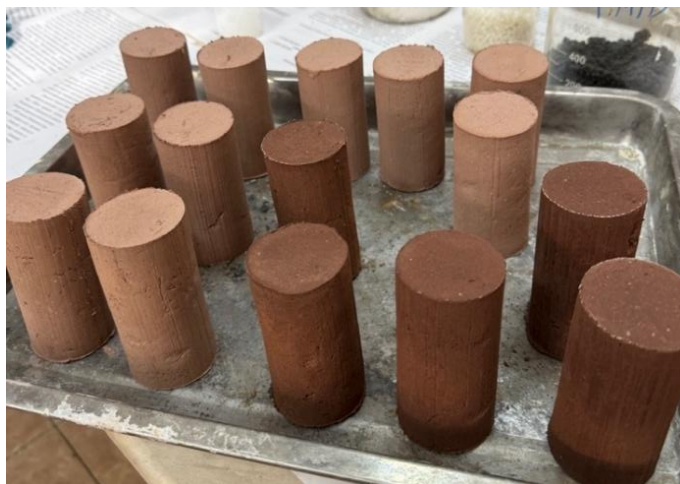
Figure 2 – Waste-based ceramic samples after drying
