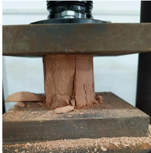
Figure 2 – Compression test of samples
