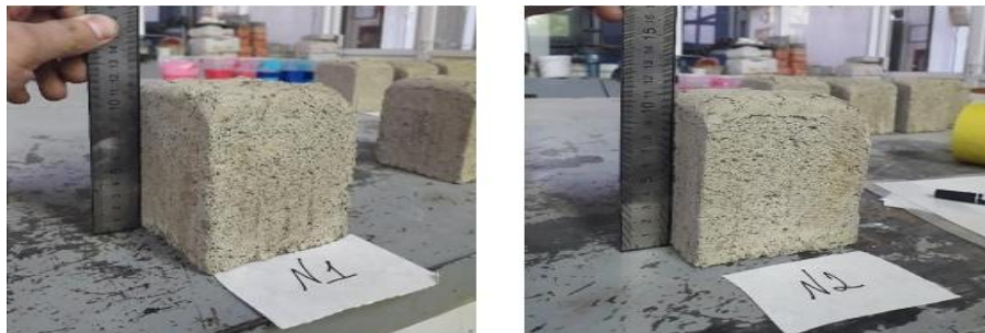
Figure 6 – Fragments of sedimentation measurements of porous samples after drying
