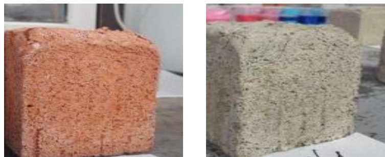
a) After drying, before firing b) After firing at t = 950\text{ }^{\circ}\text{C}
