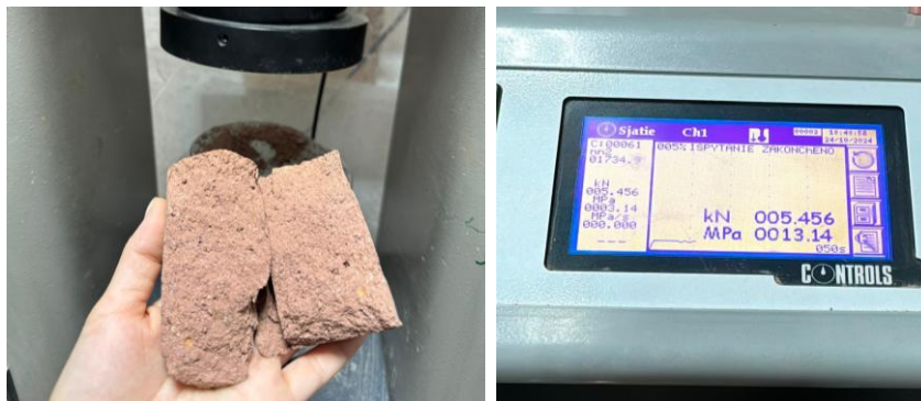
Figure 2 – Ceramic sample tested for compressive strength
