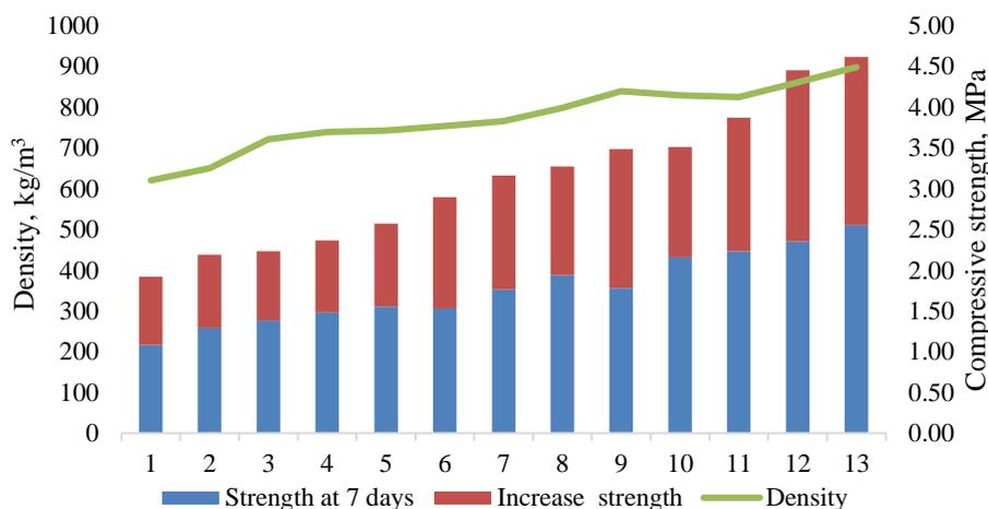
Figure 6 – Strength change histogram and density graph
