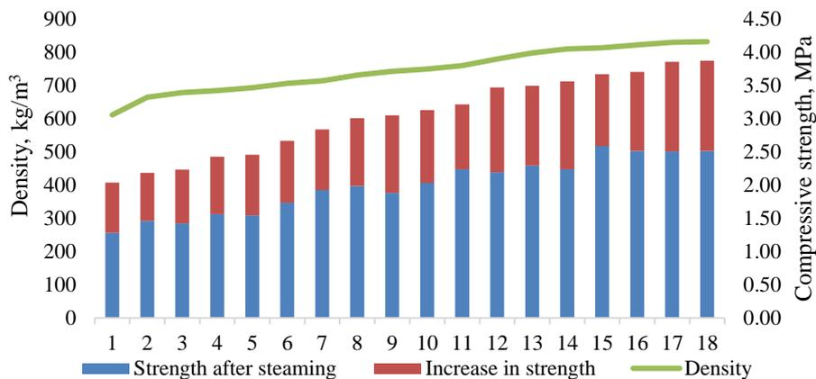
Figure 3 – Histogram of strength increase and density plot
