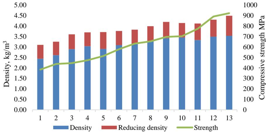
Figure 7 – Histogram of density change and strength graph
