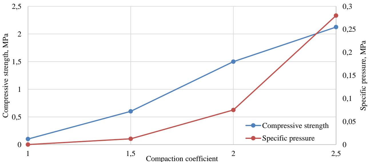
Figure 3 – The influence of the compaction coefficient on the strength of arbolite and on the specific compaction pressure of the mixture
