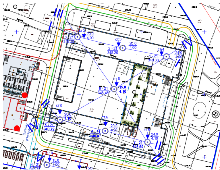
Figure 1 – Topographic survey of the construction site [14]
