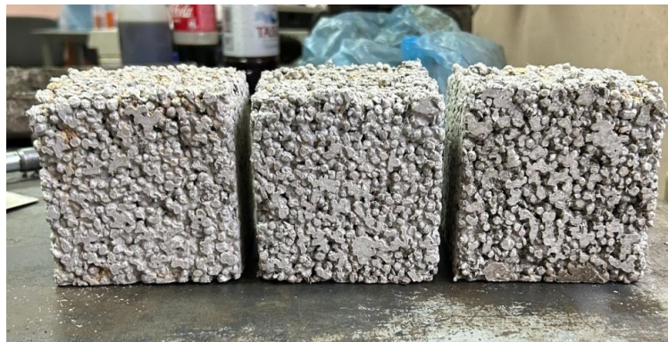
Figure 2 – Polystyrene concrete samples for research
