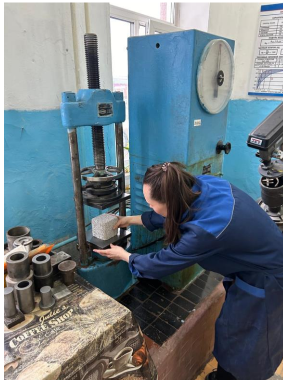
Figure 5 – Mechanical compressive strength test
