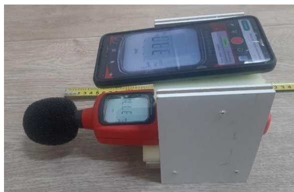
Figure 4 – Placement of the noise meter on the rack
