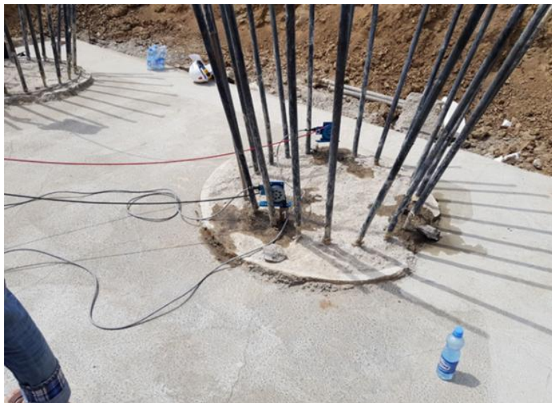
Figure 5 – CSL pile testing with two probes
