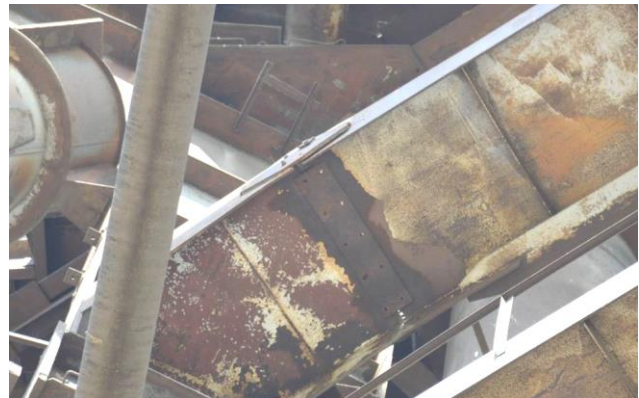
Figure 7 – Fracture of the weld at the fusion boundary along the entire length of the joint
