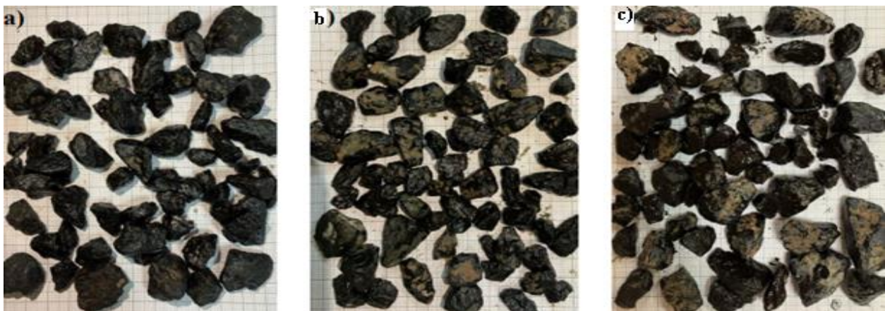
Figure 5 – The surface area of crushed stone with bitumen as a result of the decomposition of bitumen emulsion: a) without additives; b) with ZSHO Pavlodar CHP-2; c) with ZSHO Pavlodar CHP-3
