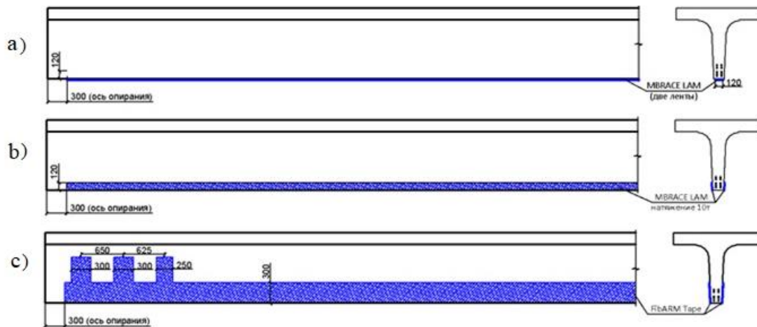
Figure 7 – Beam strengthening with composite materials: a – according to scheme 1; b – according to scheme 2; c – according to scheme 3
