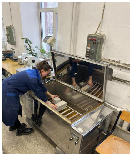
Figure 3 – Preparation of samples for steaming
