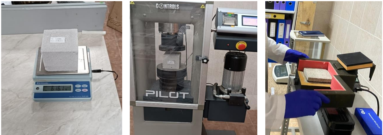
Figure 1 – Laboratory testing of foam concrete
