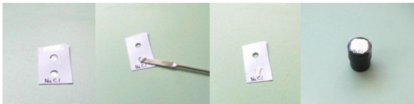
a) sample preparation b) adding the powder c) making the surface smoother d) attaching the diaphragm tube
