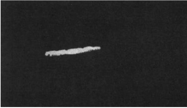
Figure 6 – Track produced by an \alpha – particle
