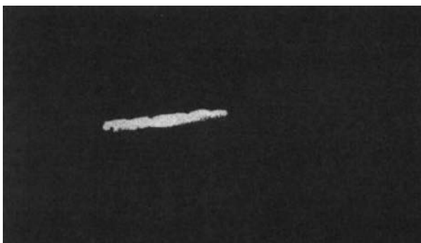
Figure 6 – Track produced by an \alpha – particle
